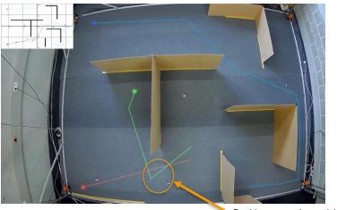
Position error when relying on LPS and Flow-deck v2
