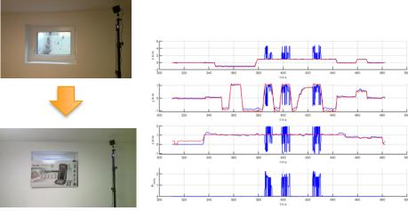
Windows causing reflections distorting Lighthouse crossing beam method
